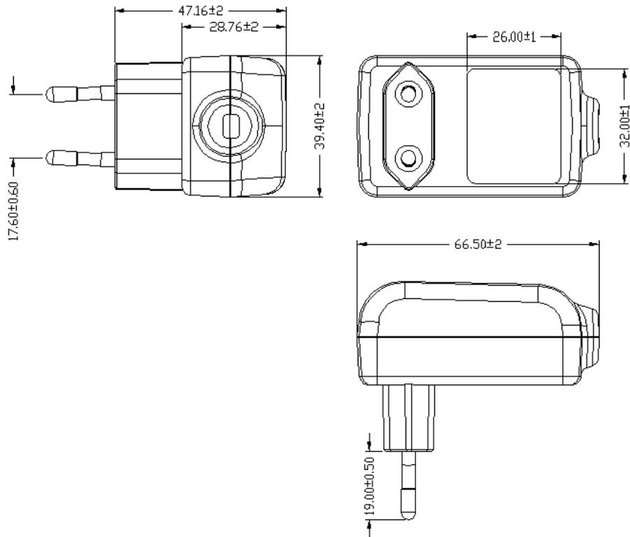
Enclosure Type: PC Temperature:  $120^{\circ}\text{C}$
